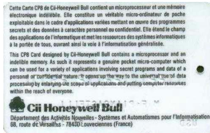
Figure 2. The Bull CP8, the first microprocessor card (1979)
